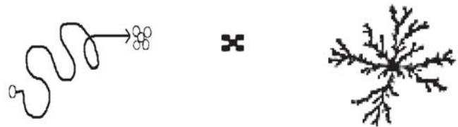
Fig. 4. Schematic diagram of Diffusion Limited Aggregation process
