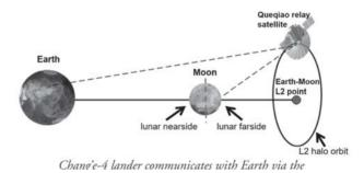
Chang'e-4 lander communicates with Earth via the Queqiao relay satellite placed at Lagrange point L2.
