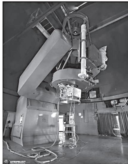
The PARAS spectrograph was designed and developed by the members of the Astronomy and Astrophysics Division of PRL. The primary aim of PARAS is to search for planets around dwarf mainsequence stars. It has wavelength coverage of 400 nm to 680 nm. (Credit: PRL)
