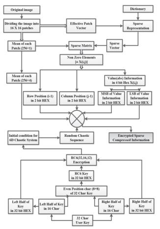
Fig. 1. Block diagram of the encryption technique.
