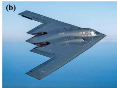
Fig. 2: Stealthy aircrafts developed through shaping: (a) F-117 and (b) B-2 Spirit. [Source: Wikipedia].
