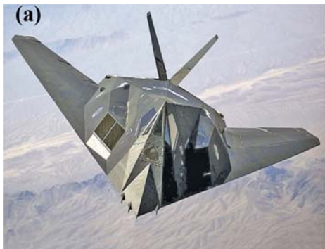
Fig. 2: Stealthy aircrafts developed through shaping: (a) F-117 and (b) B-2 Spirit. [Source: Wikipedia].
