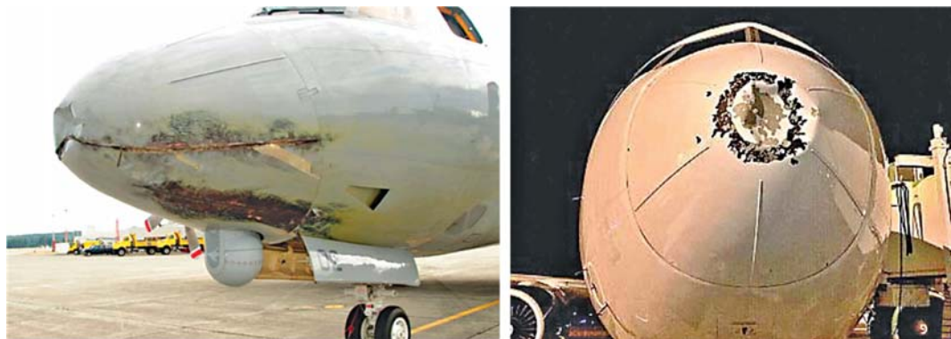
Fig. 6(a): Damages caused by lightning strike on aircraft (Courtesy: https://www.theatlantic.com & http://www.chinaaviationdaily.com/news/44/44306.html )
