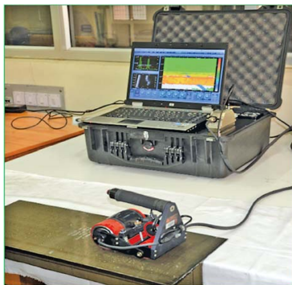
Fig. 2: Pulse echo linear Array Roller Probe (Rapid Scan System) deployed at CSIR-NAL
