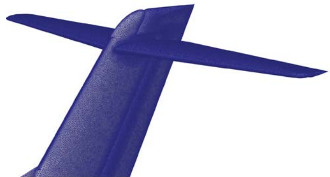
Fig. 11: CFD mesh used on HT and VT surfaces of in a zoomed view
