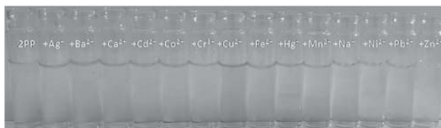
Fig. 1 (a) The color changes of 2PP (50 mM) upon addition of various aqueous cations (1 equiv.) in MeCN medium.
