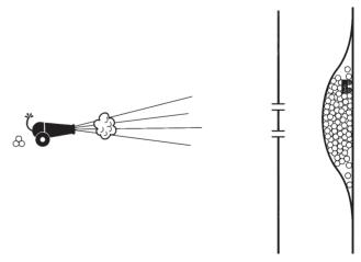
**Illustration 2.1 :** Electrons or small bullets are fired into a wall with two slits [illustration by Isabelle Zaoui]
