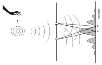
**Illustration 2.2 :** A wave is formed at left, then the wave is split into two sub-waves that interfere at the wall [Illustration by Isabelle Zaoui]
