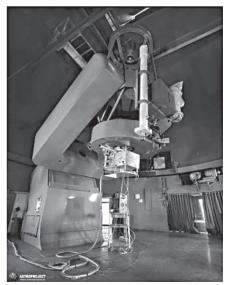
The PARAS spectrograph was designed and developed by the members of the Astronomy and Astrophysics Division of PRL. The primary aim of PARAS is to search for planets around dwarf mainsequence stars. It has wavelength coverage of 400 nm to 680 nm. (Credit: PRL)
